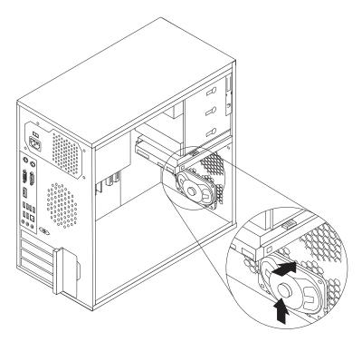
Figure 35. Removing the old internal speaker
